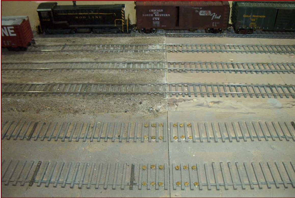
Figure 6 A submodule joint showing numerous tracks. Those closest to the foreground have brass screws. In the background there are tracks that have been laid and screws painted (right) as well as tracks that are fully scened with ballast.
