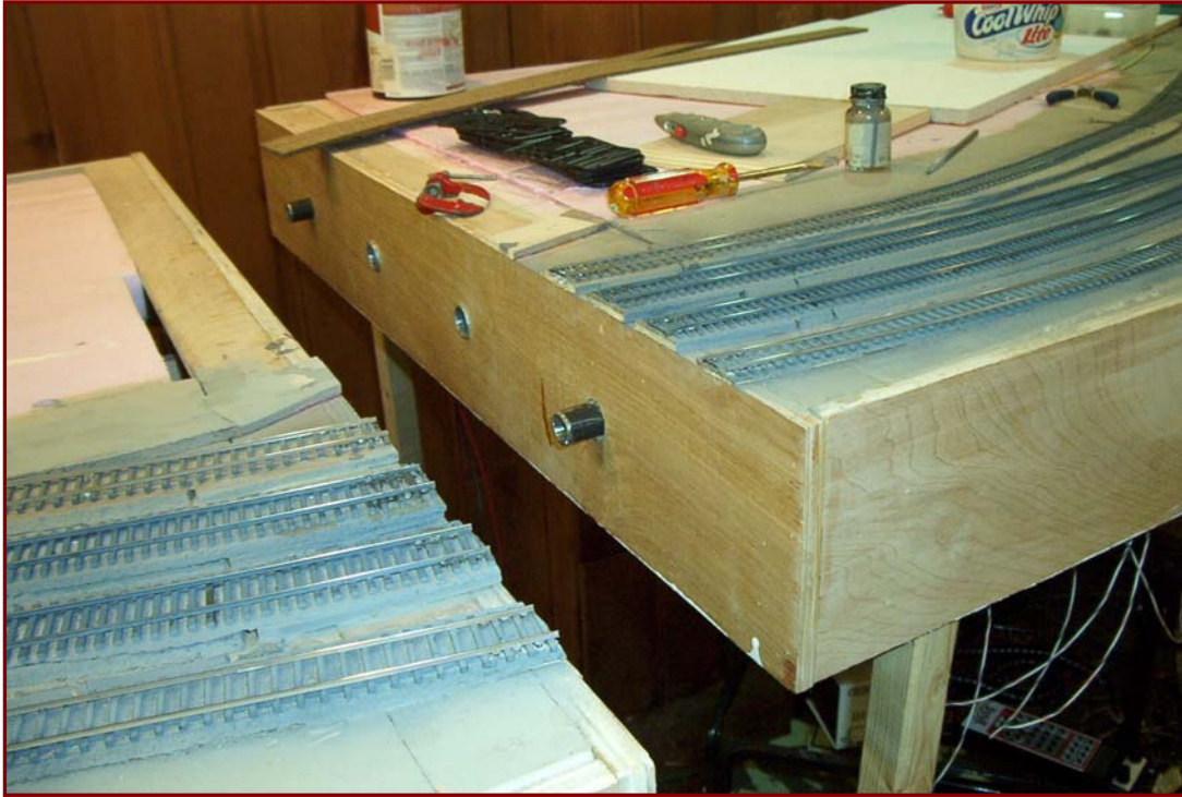
Figure 5. Intermodule joint showing installed pins and sleeves and four sets of tracks bridging the joint. Note that even curved tracks can cross the joint smoothly.
