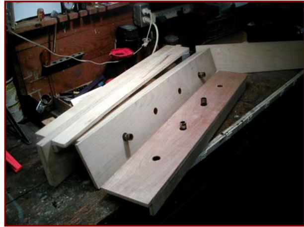
Figure 1 Two pairs of endplates with pins (one opened, one closed). In the background is a single endplate without pins.
